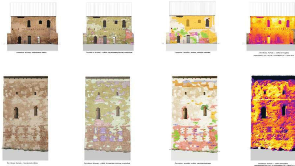
Fig. 5 - Synoptic plans: a) photogrammetric survey; b) material study; c) pathologies; d) thermography
