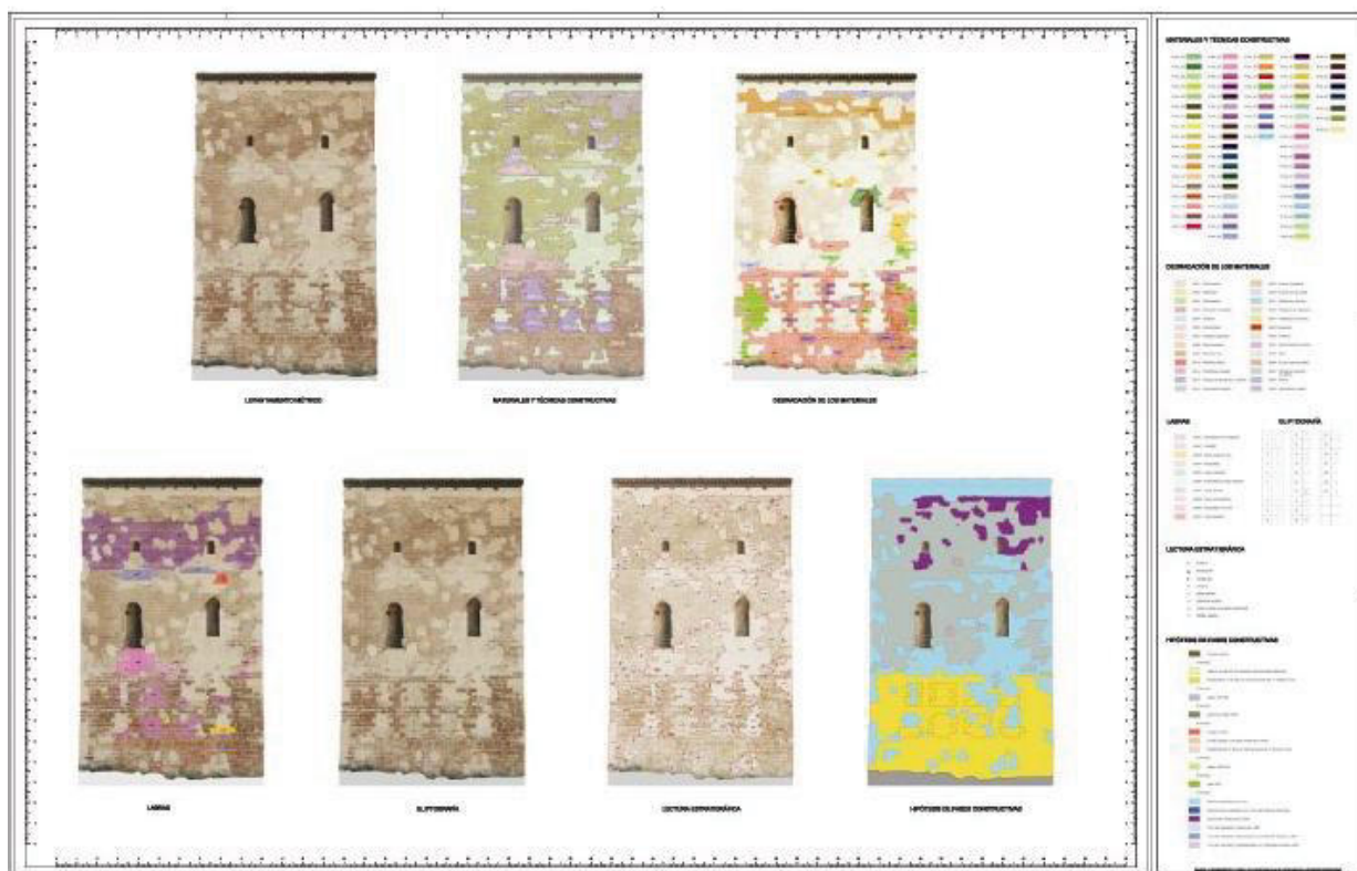
Fig. 4 - Synoptic plan of the various approaches used: photogrammetric survey (a), material study (b), pathologies (c), stonework (d), glyptography (e) and stratigraphy (f and g)
