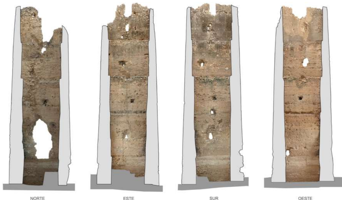
Fig. 2. Bofilla Tower, inner sections, before the conservation work (C. Mileto and F. Vegas).
