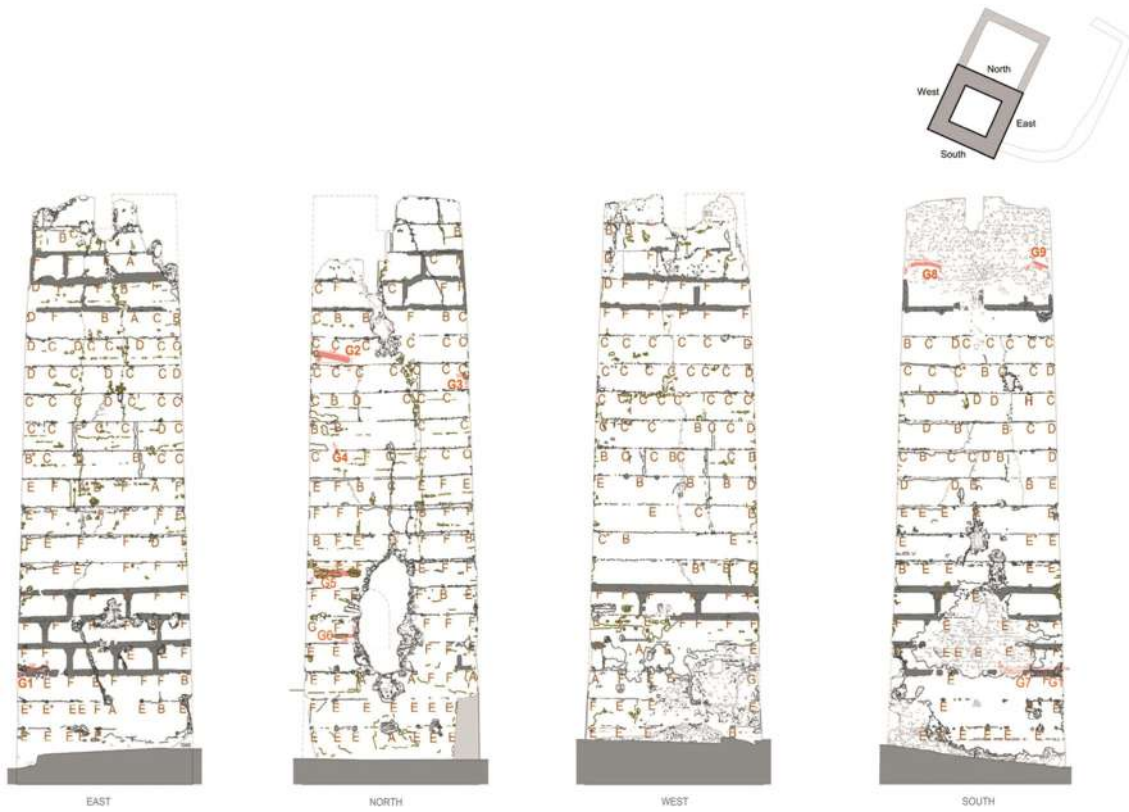
Fig. 15. Mapping of the wooden putlogs and the reinforcement in the walls of the Bofilla Tower (C. Mileto and F. Vegas).
