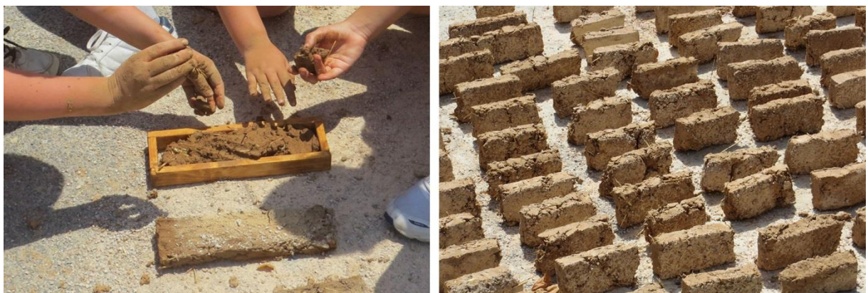
Fig. 3. Image of the adobe bricks manufactured during the workshop
