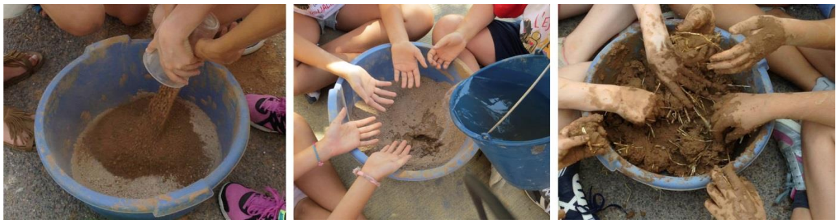
Fig. 2. Preparing the mix for manufacturing adobe.
