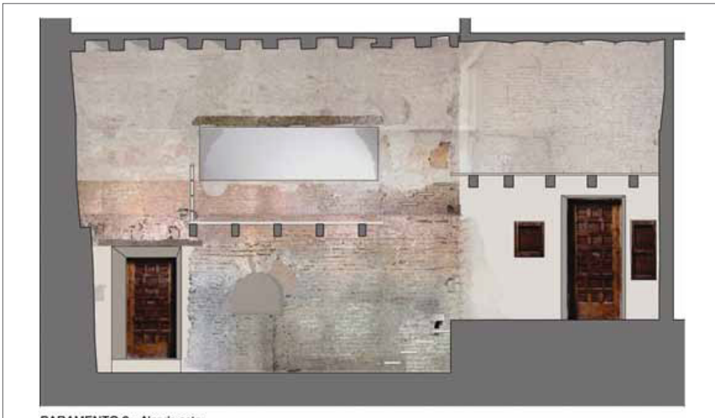
Fig. 3b Antechamber of the Mexuar in the Alhambra (Granada, Spain). Computer simulation of photoplan of elevation no.1 after restoration
