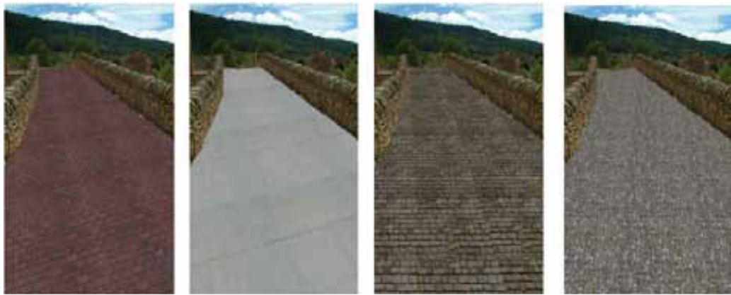
Fig. 4 Medieval bridge in Poble de Ballestar in Castellón (Spain). Several computer options done to test the impact of different ways to substitute the remains of the pavement
