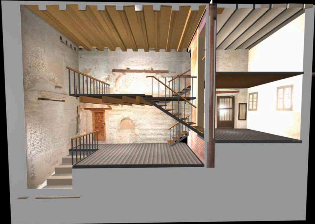
Fig. 1 Antechamber of the Mexuar in the Alhambra (Granada, Spain). Three-dimensional computer simulation of the previewed result both of the restoration of the historical surfaces and the insertion of new floors.
